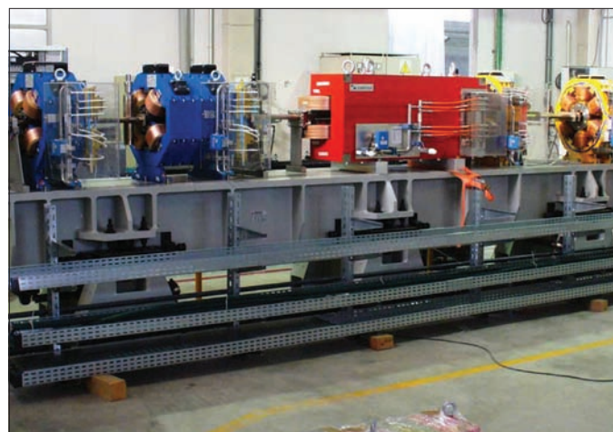
A lattice cell being prepared for ALBA's storage ring, with quadrupoles, dipoles and sextupoles. (Photos courtesy CELLS.)
